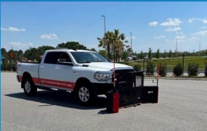
Automated debris removal system. (Source: Enforcement Engineering, Inc.)
