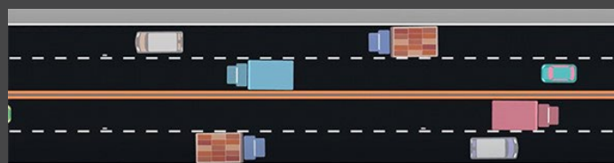
TTI analyzed cross sections on Texas roadways, including four-lane undivided roads with a centerline stripe.
